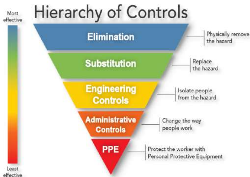
Figure 3: Hierarchy of Hazard Controls. Image Source: "Chemical Safety Training Course Material" downloaded from https://www.uab.edu/ehs/images/docs/chem/CS101-course-material.pdf
